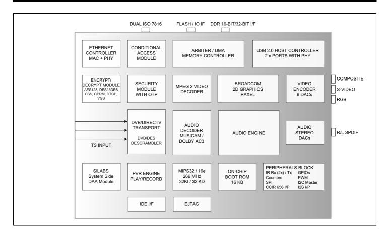
The BCM7318 is a fully integrated MPEG2 single-chip solution targeted specifically at the emerging IP-STB market.
